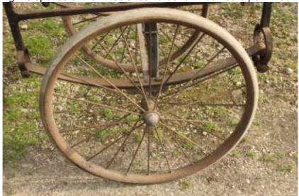
During the cleaning operation it was found that the wheels had brass hub and oil caps. Brass and bright steel parts were polished while the rim and spokes had two coats of rust protecting paint applied.
